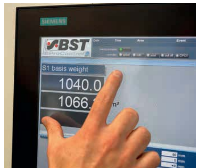
INDICON-XL is the name of BST ProControl's comfortably-operated software for realtime recording, evaluation and visualisation on a screen of measurement results in the form of cross and longitudinal sections.
